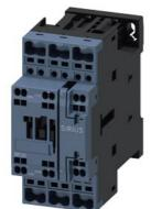
power contactor, AC-3e/AC-3, 9 A, 4 kW / 400 V, 3-pole, 110 V AC, 50 Hz / 120 V, 60 Hz, auxiliary contacts: 1 NO + 1 NC, spring-loaded terminal, size: S0
