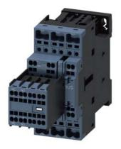
power contactor, AC-3e/AC-3, 9 A, 4 kW / 400 V, 3-pole, 110 V AC, 50/60 Hz, auxiliary contacts: 2 NO + 2 NC, spring-loaded terminal, size: S0, removable auxiliary switch
