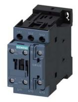
power contactor, AC-3e/AC-3, 9 A, 4 kW / 400 V, 3-pole, 24 V DC, with plugged-in diode combination, auxiliary contacts: 1 NO + 1 NC, screw terminal, size: S0  $\,$
