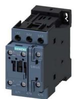
power contactor, AC-3e/AC-3, 9 A, 4 kW / 400 V, 3-pole, 24 V DC, auxiliary contacts: 1 NO + 1 NC, screw terminal, size: S0, communication-capable
