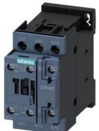
power contactor, AC-3e/AC-3, 9 A, 4 kW / 400 V, 3-pole, 220 V AC, 50 Hz / 240 V, 60 Hz, auxiliary contacts: 1 NO + 1 NC, screw terminal, size: S0
