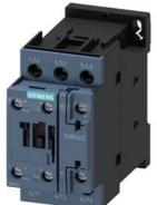
power contactor, AC-3e/AC-3, 9 A, 4 kW / 400 V, 3-pole, 110 V AC, 50 Hz / 120 V, 60 Hz, auxiliary contacts: 1 NO + 1 NC, screw terminal, size: S0
