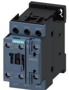
power contactor, AC-3e/AC-3, 9 A, 4 kW / 400 V, 3-pole, 24 V AC, 50/60 Hz, auxiliary contacts: 1 NO + 1 NC, screw terminal, size: S0
