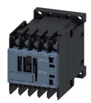
power contactor, AC-3e/AC-3, 16 A, 7.5 kW / 400 V, 3-pole, 24 V DC, auxiliary contacts: 1 NC, ring cable lug connection, size: S00  $\,$
