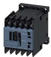
power contactor, AC-3e/AC-3, 16 A, 7.5 kW / 400 V, 3-pole, 400 V AC, 50 Hz / 400-440 V, 60 Hz, auxiliary contacts: 1 NC, ring cable lug connection, size: S00
