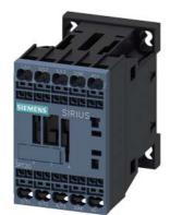
power contactor, AC-3e/AC-3, 16 A, 7.5 kW / 400 V, 3-pole, 24 V DC, with integrated diode, auxiliary contacts: 1 NC, spring-loaded terminal, size: S00
