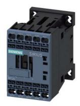
power contactor, AC-3e/AC-3, 16 A, 7.5 kW / 400 V, 3-pole, 24 V DC, auxiliary contacts: 1 NC, spring-loaded terminal, size: S00  $\,$
