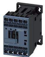
power contactor, AC-3e/AC-3, 16 A, 7.5 kW / 400 V, 3-pole, 24 V DC, auxiliary contacts: 1 NC, spring-loaded terminal, size: S00, communication-capable
