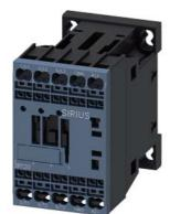
power contactor, AC-3e/AC-3, 16 A, 7.5 kW / 400 V, 3-pole, 24 V DC, auxiliary contacts: 1 NO, spring-loaded terminal, size: S00, communication-capable
