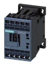
power contactor, AC-3e/AC-3, 16 A, 7.5 kW / 400 V, 3-pole, 48 V AC, 50/60 Hz, auxiliary contacts: 1 NC, spring-loaded terminal, size: S00
