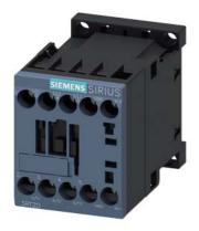
contactor, NEMA version, 5 HP, 460 / 575 V, 3-pole, 24 V DC, auxiliary contacts: 1 NO, screw terminal, size:  $\rm S00$
