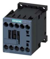
contactor, NEMA version, 5 HP, 460 / 575 V, 3-pole, 480 V AC, 60 Hz, auxiliary contacts: 1 NO, screw terminal, size: S00  $\,$
