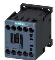
power contactor, AC-3e/AC-3, 16 A, 7.5 kW / 400 V, 3-pole, 110 V AC, 50 Hz / 120 V, 60 Hz, auxiliary contacts: 1 NO, screw terminal, size: S00
