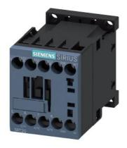
power contactor, AC-3e/AC-3, 16 A, 7.5 kW / 400 V, 3-pole, 48 V AC, 50/60 Hz, auxiliary contacts: 1 NC, screw terminal, size: S00  $\,$
