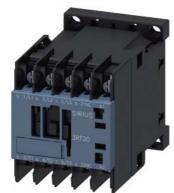
power contactor, AC-3e/AC-3, 12 A, 5.5 kW / 400 V, 3-pole, 400 V AC, 50 Hz / 400-440 V, 60 Hz, auxiliary contacts: 1 NC, ring cable lug connection, size: S00
