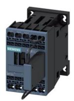
traction contactor, AC-3e/AC-3, 12 A, 5.5 kW / 400 V, 3-pole, 110 V DC, 0.7-1.25\* Us, with integrated varistor, auxiliary contacts: 1 NC, spring-loaded terminal, size: S00, with plugged on series resistor, upright mounting position
