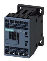
power contactor, AC-3e/AC-3, 12 A, 5.5 kW / 400 V, 3-pole, 110 V DC, 0.7-1.25  $^{\ast}$  Us, with integrated varistor, auxiliary contacts: 1 NO, spring-loaded terminal, size: S00
