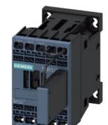
traction contactor, AC-3e/AC-3, 12 A, 5.5 kW / 400 V, 3-pole, 125 V DC, 0.7-1.25\* Us, with integrated suppressor diode, auxiliary contacts: 1 NC, spring-loaded terminal, size: S00, with plugged on series resistor
