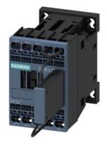
traction contactor, AC-3e/AC-3, 12 A, 5.5 kW / 400 V, 3-pole, 110 V DC, 0.7-1.25  $^{\star}$  Us, with integrated suppressor diode, auxiliary contacts: 1 NC, spring-loaded terminal, size: S00, with plugged on series resistor, upright mounting position
