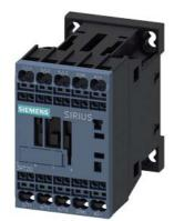
power contactor, AC-3e/AC-3, 12 A, 5.5 kW / 400 V, 3-pole, 24 V DC, 0.7-1.25\* Us, with integrated suppressor diode, auxiliary contacts: 1 NC, spring-loaded terminal, size: S00, suitable for PLC outputs, not expandable with auxiliary switch
