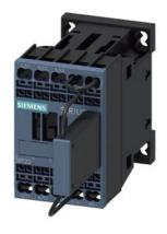
traction contactor, AC-3e/AC-3, 12 A, 5.5 kW / 400 V, 3-pole, 24 V DC, 0.7-1.25  $^{\star}$  Us, with integrated suppressor diode, auxiliary contacts: 1 NC, spring-loaded terminal, size: S00, suitable for PLC outputs, not expandable with auxiliary switch , upright mounting position
