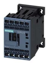
power contactor, AC-3e/AC-3, 12 A, 5.5 kW / 400 V, 3-pole, 24 V DC, 0.7-1.25\* Us, with integrated suppressor diode, auxiliary contacts: 1 NO, spring-loaded terminal, size: S00, suitable for PLC outputs, not expandable with auxiliary switch
