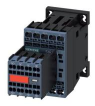
power contactor, AC-3e/AC-3, 12 A, 5.5 kW / 400 V, 3-pole, 24 V DC, auxiliary contacts: 2 NO + 2 NC, spring-loaded terminal, size: S00, captive auxiliary switch
