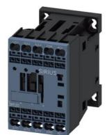
power contactor, AC-3e/AC-3, 12 A, 5.5 kW / 400 V, 3-pole, 24 V DC, auxiliary contacts: 1 NC, spring-loaded terminal, size: S00, communication-capable
