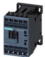
power contactor, AC-3e/AC-3, 12 A, 5.5 kW / 400 V, 3-pole, 220 V AC, 50 Hz / 240 V, 60 Hz, auxiliary contacts: 1 NC, spring-loaded terminal, size: S00  $\,$
