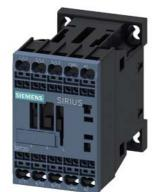
power contactor, AC-3e/AC-3, 12 A, 5.5 kW / 400 V, 3-pole, 24 V AC, 50/60 Hz, auxiliary contacts: 1 NO, spring-loaded terminal, size: S00  $\,$
