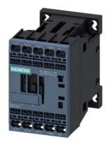
power contactor, AC-3e/AC-3, 12 A,  $5.5\,\mathrm{kW}$  / 400 V, 3-pole, 24 V AC, 50/60 Hz, auxiliary contacts: 1 NO, spring-loaded terminal, size: S00, upright mounting position
