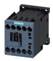
power contactor, AC-3e/AC-3, 12 A, 5.5 kW / 400 V, 3-pole, 24 V DC, 0.85-1.85  $^{\star}$  Us, auxiliary contacts: 1 NO, screw terminal, size: S00, not expandable with auxiliary switch
