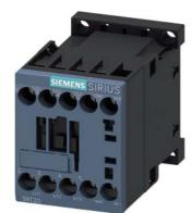
power contactor, AC-3e/AC-3, 12 A, 5.5 kW / 400 V, 3-pole, 24 V DC, 0.7-1.25\* Us, with integrated diode, auxiliary contacts: 1 NO, screw terminal, size: S00, suitable for PLC outputs, not expandable with auxiliary switch
