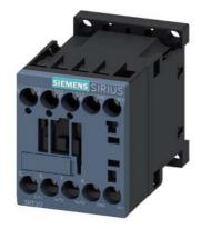
power contactor, AC-3e/AC-3, 12 A, 5.5 kW / 400 V, 3-pole, 24 V DC, auxiliary contacts: 1 NC, screw terminal, size: S00, communication-capable
