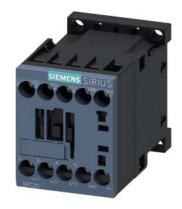
power contactor, AC-3e/AC-3, 12 A, 5.5 kW / 400 V, 3-pole, 24 V DC, auxiliary contacts: 1 NO, screw terminal, size: S00  $\,$
