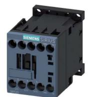
power contactor, AC-3e/AC-3, 12 A, 5.5 kW / 400 V, 3-pole, 220 V AC, 50 Hz / 240 V, 60 Hz, auxiliary contacts: 1 NO, screw terminal, size: S00
