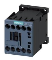
power contactor, AC-3e/AC-3, 12 A, 5.5 kW / 400 V, 3-pole, 230 V AC, 50/60 Hz, auxiliary contacts: 1 NC, screw terminal, size: S00, upright mounting position
