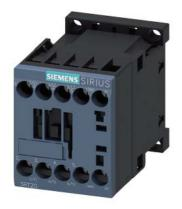
power contactor, AC-3e/AC-3, 12 A, 5.5 kW / 400 V, 3-pole, 230 V AC, 50/60 Hz, auxiliary contacts: 1 NO, screw terminal, size: S00  $\,$
