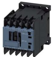
power contactor, AC-3e/AC-3, 9 A, 4 kW / 400 V, 3-pole, 220 V AC, 50 Hz / 240 V, 60 Hz, auxiliary contacts: 1 NC, ring cable lug connection, size: S00
