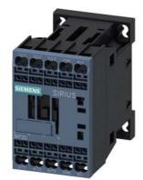
power contactor, AC-3e/AC-3, 9 A, 4 kW / 400 V, 3-pole, 24 V DC, 0.7-1.25\* Us, auxiliary contacts: 1 NC, spring-loaded terminal, size: S00, suitable for PLC outputs, not expandable with auxiliary switch
