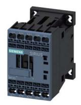
power contactor, AC-3e/AC-3, 9 A, 4 kW / 400 V, 3-pole, 24 V DC, with integrated diode, auxiliary contacts: 1 NC, spring-loaded terminal, size: S00  $\,$
