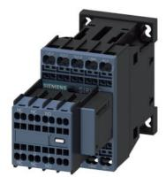
power contactor, AC-3e/AC-3, 9 A, 4 kW / 400 V, 3-pole, 24 V DC, with varistor plugged on, auxiliary contacts: 2 NO + 2 NC, spring-loaded terminal, size: S00, removable auxiliary switch
