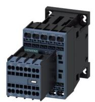
power contactor, AC-3e/AC-3, 9 A, 4 kW / 400 V, 3-pole, 24 V DC, auxiliary contacts: 2 NO + 2 NC, spring-loaded terminal, size: S00, removable auxiliary switch
