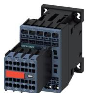
power contactor, AC-3e/AC-3, 9 A, 4 kW / 400 V, 3-pole, 24 V DC, auxiliary contacts: 2 NO + 2 NC, spring-loaded terminal, size: S00, captive auxiliary switch
