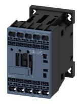
power contactor, AC-3e/AC-3, 9 A, 4 kW / 400 V, 3-pole, 24 V DC, auxiliary contacts: 1 NC, spring-loaded terminal, size: S00, communication-capable
