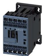
power contactor, AC-3e/AC-3, 9 A, 4 kW / 400 V, 3-pole, 24 V DC, auxiliary contacts: 1 NO, spring-loaded terminal, size: S00, communication-capable
