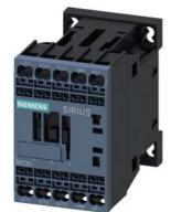
power contactor, AC-3e/AC-3, 9 A, 4 kW / 400 V, 3-pole, 12 V DC, auxiliary contacts: 1 NO, spring-loaded terminal, size: S00  $\,$
