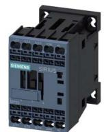
power contactor, AC-3e/AC-3, 9 A, 4 kW / 400 V, 3-pole, 220 V AC, 50 Hz / 240 V, 60 Hz, auxiliary contacts: 1 NC, spring-loaded terminal, size: S00  $\,$
