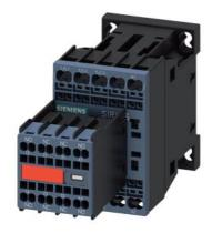
power contactor, AC-3e/AC-3, 9 A, 4 kW / 400 V, 3-pole, 110 V AC, 50 Hz / 120 V, 60 Hz, auxiliary contacts: 2 NO + 2 NC, spring-loaded terminal, size: S00, captive auxiliary switch
