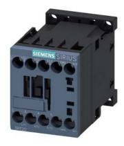
power contactor, AC-3e/AC-3, 9 A, 4 kW / 400 V, 3-pole, 24 V DC, 0.7-1.25\* Us, with integrated suppressor diode, auxiliary contacts: 1 NO, screw terminal, size: S00, suitable for PLC outputs, not expandable with auxiliary switch
